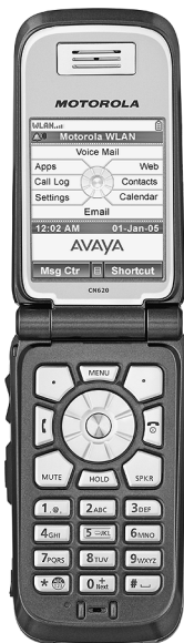
Figure II-2: An integrated cell phone/WiFi phone.
